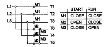
C.9 lead, Dual Voltage & Voltage Ratio 1 to 2. Wye connected.
