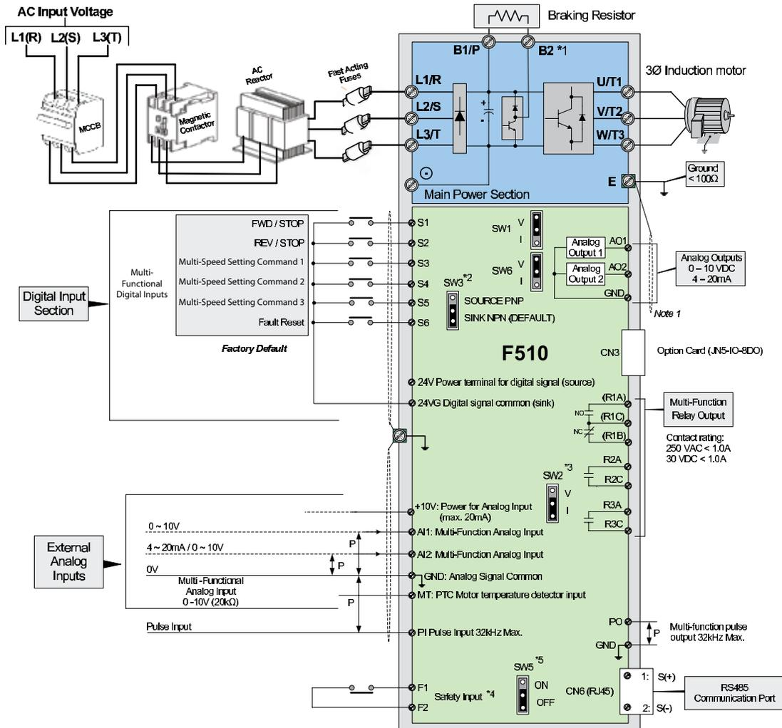
\*1 - Models that are IP20, 5-30 hp (230V) and 5-40 hp (460V), have a built-in braking transistor. To use this braking transistor, the braking resistor can be connected between terminal B1 and B2.
