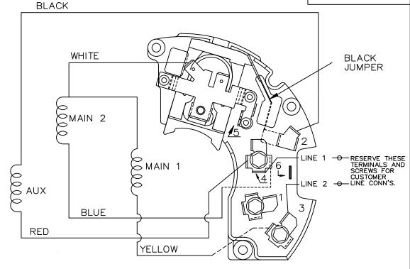
SINGLE HIGH VOLTAGE CAPACITOR START REVERSIBLE ON TERM BOARD NO OVERLOAD PROTECTION
