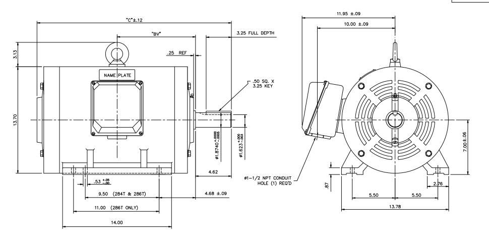
NOTE: 286T HAS 6 MTG. HOLES, USING 284T AND 286T LOCATIONS
