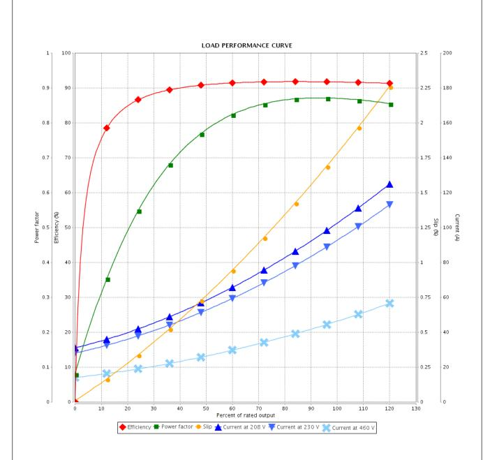
Performance : 208-230/460 V 60 Hz 2P : 104-94.4/47.2 A Rated current Moment of inertia (J) : 1.91 sq.ft.lb **LRC** Duty cycle : Cont.(S1) : 6.1 Insulation class : 58.6 ft.lb : F Rated torque Locked rotor torque : 170 % Service factor : 1.15 Breakdown torque : 250 % Temperature rise : 80 K Rated speed : 3535 rpm Design : B Rev. Performed Checked **Changes Summary** Date Performed by Checked by Revision Page
