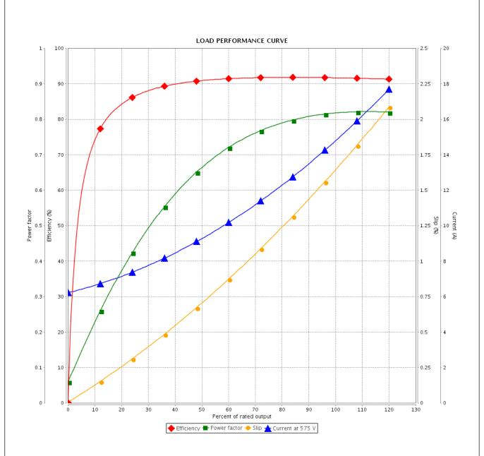
Performance : 575 V 60 Hz 6P : 14.7 A Rated current Moment of inertia (J) : 4.80 sq.ft.lb **LRC** Duty cycle : Cont.(S1) : 6.3 : 65.9 ft.lb Insulation class : F Rated torque Locked rotor torque : 260 % Service factor : 1.25 Breakdown torque : 260 % Temperature rise : 80 K Rated speed : 1180 rpm Design : B Rev. Performed Checked **Changes Summary** Date Performed by
