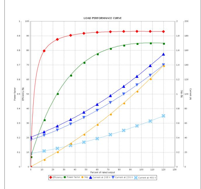
Performance : 208-230/460 V 60 Hz 2P : 130-117/58.7 A Moment of inertia (J) : 3.02 sq.ft.lb Rated current **LRC** Duty cycle : Cont.(S1) : 6.3 Insulation class : 72.8 ft.lb : F Rated torque Locked rotor torque : 200 % Service factor : 1.25 Breakdown torque : 220 % Temperature rise : 80 K Rated speed : 3560 rpm Design : B Checked Rev. **Changes Summary** Performed Date Performed by
