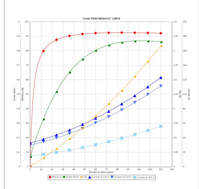
Performance : 208-230/460 V 60 Hz 2P : 104-93.6/46.8 A Moment of inertia (J) : 2.02 sq.ft.lb Rated current **LRC** : Cont.(S1) : 6.5 Duty cycle Insulation class : 58.5 ft.lb : F Rated torque Locked rotor torque : 190 % Service factor : 1.25 Breakdown torque : 260 % Temperature rise : 80 K Rated speed : 3540 rpm Design : B Rev Changes Summary Performed Checked Date
