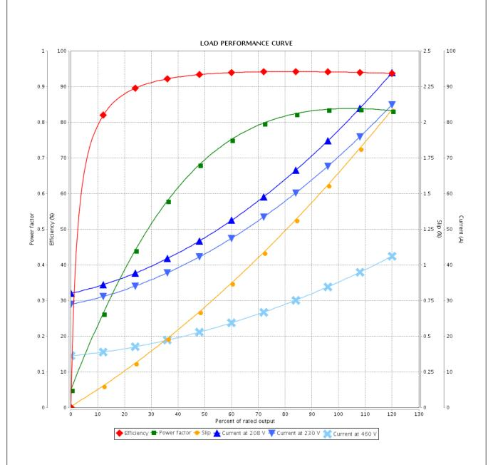
Performance : 208-230/460 V 60 Hz 4P : 77.2-69.8/34.9 A Moment of inertia (J) : 4.52 sq.ft.lb Rated current **LRC** Duty cycle : Cont.(S1) : 6.6 Insulation class : 87.8 ft.lb : F Rated torque Locked rotor torque : 280 % Service factor : 1.25 Breakdown torque : 280 % Temperature rise : 80 K Rated speed : 1770 rpm Design : B Checked Rev. Performed **Changes Summary** Date Performed by Checked by Revision Page
