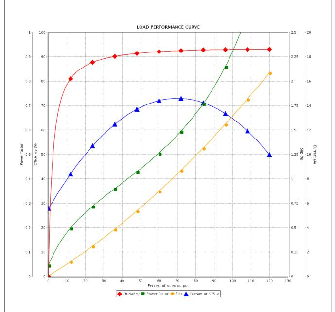
Performance : 575 V 60 Hz 4P : 14.0 A Rated current Moment of inertia (J) : 2.72 sq.ft.lb **LRC** Duty cycle : Cont.(S1) : 6.4 : 43.9 ft.lb Insulation class : F Rated torque Locked rotor torque : 240 % Service factor : 1.25 Breakdown torque : 280 % Temperature rise : 80 K Rated speed : 1770 rpm Design : B Rev. Performed Checked **Changes Summary** Date Performed by Checked by Revision Page
