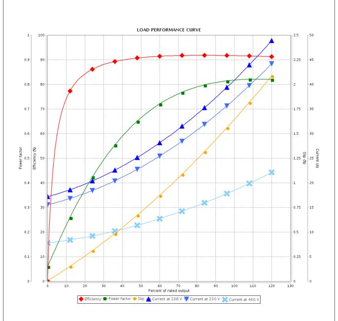
Performance : 208-230/460 V 60 Hz 6P : 40.7-36.8/18.4 A Moment of inertia (J) : 4.80 sq.ft.lb Rated current **LRC** Duty cycle : 6.3 : Cont.(S1) Insulation class : 65.9 ft.lb : F Rated torque Locked rotor torque : 260 % Service factor : 1.25 Breakdown torque : 260 % Temperature rise : 80 K Rated speed : 1180 rpm Design : B Checked Rev. Performed **Changes Summary** Date Performed by Checked by Revision Page
