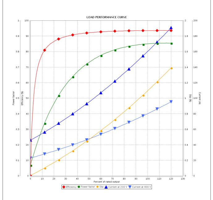
Performance : 200/400 V 60 Hz 2P : 163/81.7 A Moment of inertia (J) : 3.82 sq.ft.lb Rated current **LRC** Duty cycle : Cont.(S1) : 6.3 : 87.3 ft.lb Insulation class Rated torque : F Locked rotor torque : 220 % Service factor : 1.25 Breakdown torque : 229 % Temperature rise : 80 K Rated speed : 3560 rpm Design : B
