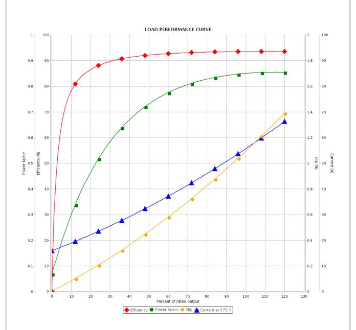
Performance : 575 V 60 Hz 2P Rated current : 56.8 A Moment of inertia (J) : 3.82 sq.ft.lb **LRC** Duty cycle : Cont.(S1) : 6.3 : 87.3 ft.lb Insulation class : F Rated torque Locked rotor torque : 220 % Service factor : 1.25 Breakdown torque : 229 % Temperature rise : 80 K Rated speed : 3560 rpm Design : B Rev. Performed Checked **Changes Summary** Date Performed by
