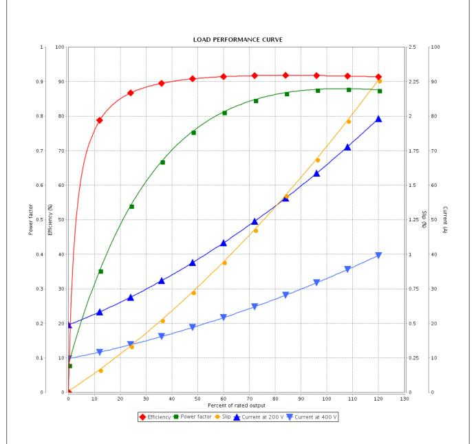
Performance : 200/400 V 60 Hz 2P Rated current : 66.2/33.1 A Moment of inertia (J) : 1.13 sq.ft.lb **LRC** Duty cycle : Cont.(S1) : 6.5 : 36.6 ft.lb Insulation class : F Rated torque Locked rotor torque : 200 % Service factor : 1.25 Breakdown torque : 280 % Temperature rise : 80 K Rated speed : 3535 rpm Design : B Rev. Performed Checked **Changes Summary** Date Performed by
