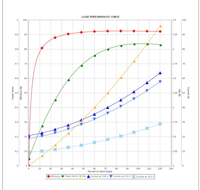
Performance : 208-230/460 V 60 Hz 6P : 53.7-48.6/24.3 A Moment of inertia (J) : 6.89 sq.ft.lb Rated current **LRC** Duty cycle : 6.4 : Cont.(S1) Insulation class : 88.0 ft.lb : F Rated torque Locked rotor torque : 229 % Service factor : 1.25 Breakdown torque : 260 % Temperature rise : 80 K Rated speed : 1177 rpm Design : B Checked Rev. **Changes Summary** Performed Date Performed by
