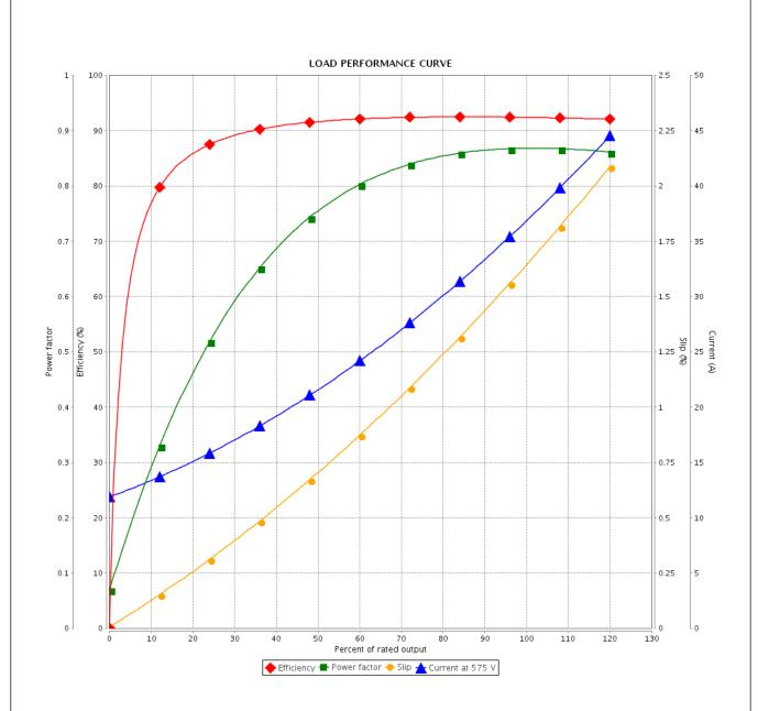
Performance : 575 V 60 Hz 2P Rated current : 37.4 A Moment of inertia (J) : 2.02 sq.ft.lb **LRC** Duty cycle : Cont.(S1) : 6.5 : 58.5 ft.lb Insulation class Rated torque : F Locked rotor torque : 190 % Service factor : 1.25 Breakdown torque : 260 % Temperature rise : 80 K Rated speed : 3540 rpm Design : B Rev. Checked **Changes Summary** Performed Date
