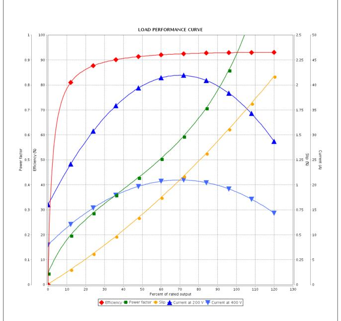
Performance : 200/400 V 60 Hz 4P Rated current : 40.2/20.1 A Moment of inertia (J) : 2.72 sq.ft.lb **LRC** Duty cycle : Cont.(S1) : 6.4 : 43.9 ft.lb Insulation class Rated torque : F Locked rotor torque : 240 % Service factor : 1.25 Breakdown torque : 280 % Temperature rise : 80 K Rated speed : 1770 rpm Design : B Rev Changes Summary Performed Checked Date
