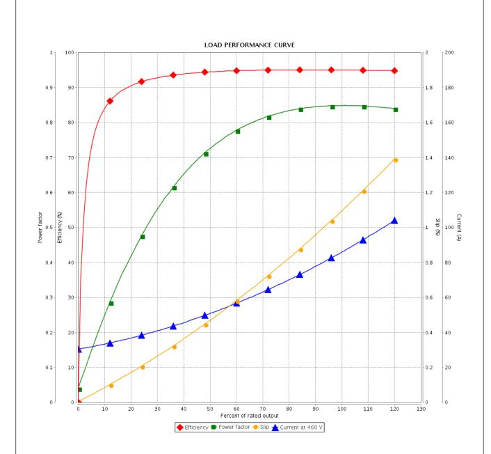
Performance : 460 V 60 Hz 4P : 85.5 A Moment of inertia (J) : 16.8 sq.ft.lb Rated current **LRC** : 6.8 Duty cycle : Cont.(S1) Insulation class : 218 ft.lb : F Rated torque Locked rotor torque : 220 % Service factor : 1.25 Breakdown torque : 260 % Temperature rise : 80 K Rated speed : 1780 rpm Design : B
