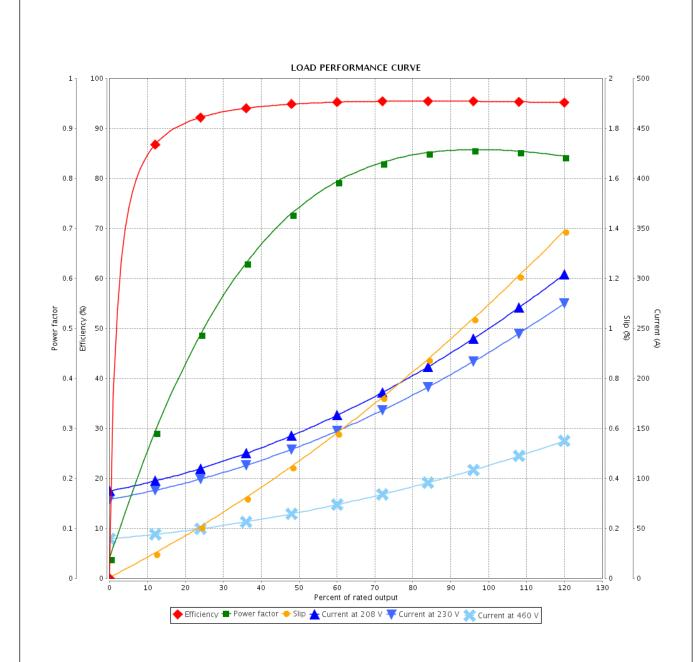
Performance : 208-230/460 V 60 Hz 4P : 254-230/115 A Moment of inertia (J) : 21.9 sq.ft.lb Rated current **LRC** Duty cycle : Cont.(S1) : 6.8 Insulation class : 291 ft.lb : F Rated torque Locked rotor torque : 200 % Service factor : 1.25 Breakdown torque : 250 % Temperature rise : 80 K Rated speed : 1780 rpm Design : B Checked Rev. Performed **Changes Summary** Date Performed by Checked by Revision Page
