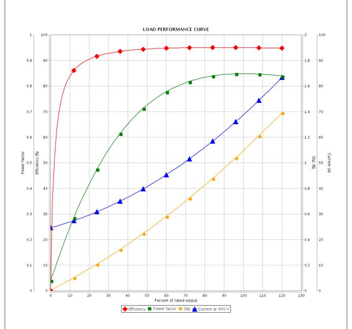
Performance : 460 V 60 Hz 4P Rated current : 69.9 A Moment of inertia (J) : 15.6 sq.ft.lb **LRC** Duty cycle : Cont.(S1) : 6.5 Insulation class : 175 ft.lb : F Rated torque Locked rotor torque : 200 % Service factor : 1.25 Breakdown torque : 240 % Temperature rise : 80 K Rated speed : 1780 rpm Design : B Rev. Performed Checked **Changes Summary** Date Performed by
