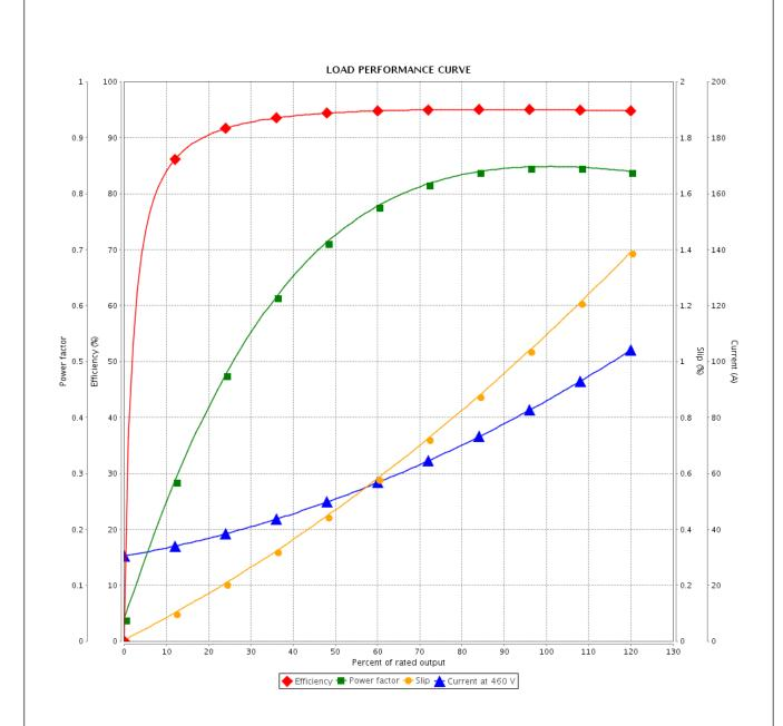
Performance : 460 V 60 Hz 4P : 85.5 A Moment of inertia (J) : 16.8 sq.ft.lb Rated current **LRC** Duty cycle : 6.8 : Cont.(S1) Insulation class : 218 ft.lb : F Rated torque Locked rotor torque : 220 % Service factor : 1.25 Breakdown torque : 260 % Temperature rise : 80 K Rated speed : 1780 rpm Design : B Checked Rev. Performed **Changes Summary** Date Performed by
