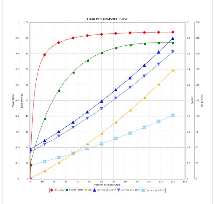
Performance : 208-230/460 V 60 Hz 2P : 188-170/84.8 A Moment of inertia (J) : 6.40 sq.ft.lb Rated current **LRC** Duty cycle : 6.6 : Cont.(S1) Insulation class : 109 ft.lb : F Rated torque Locked rotor torque : 200 % Service factor : 1.25 Breakdown torque : 250 % Temperature rise : 80 K Rated speed : 3560 rpm Design : B Checked Rev. **Changes Summary** Performed Date Performed by Checked by Revision Page
