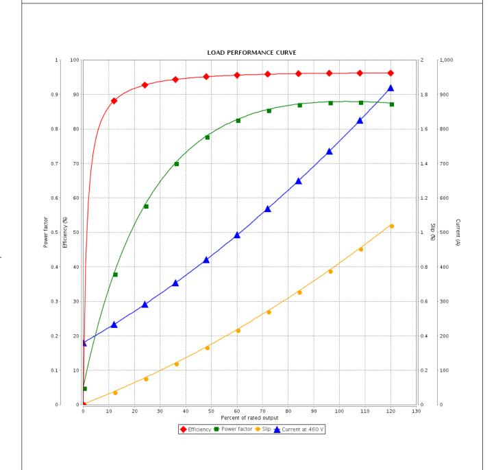
Performance : 460 V 60 Hz 2P : 764 A Rated current Moment of inertia (J) : 78.5 sq.ft.lb **LRC** : 6.8 Duty cycle : Cont.(S1) : 1020 ft.lb Insulation class Rated torque : F Locked rotor torque : 200 % Service factor : 1.15 Breakdown torque : 240 % Temperature rise : 105 K
