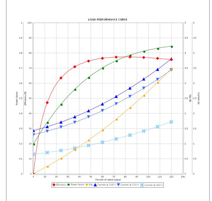
Performance : 208-230/460 V 60 Hz 2P Rated current : 3.13-2.98/1.49 A Moment of inertia (J) : 0.0415 sq.ft.lb **LRC** : 9.0 Duty cycle : Cont.(S1) Insulation class : F Rated torque : 1.48 ft.lb Locked rotor torque : 340 % Service factor : 1.15 Breakdown torque : 400 % Temperature rise : 80 K Rated speed : 3500 rpm Design : B Performed Checked Rev. **Changes Summary** Date Performed by
