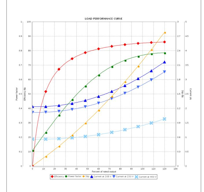
Performance : 208-230/460 V 60 Hz 4P : 3.16-2.86/1.43 A Moment of inertia (J) : 0.0975 sq.ft.lb Rated current **LRC** Duty cycle : Cont.(S1) : 8.6 : F Rated torque : 2.94 ft.lb Insulation class Locked rotor torque : 290 % Service factor : 1.15 Breakdown torque : 370 % Temperature rise : 80 K Rated speed : 1760 rpm Design : B
