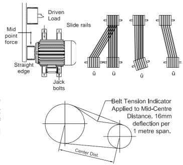
As a general rule the midpoint of the applied force should be at the midpoint of the shaft and it is good engineering practice to mount the motor pulley with hub and locking screw at the shaft end.
