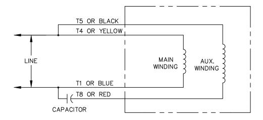
CONNECTIONS SHOWN FOR CCW ROTATION FACING LEAD END.
