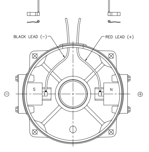
EXTERNAL CONNECTIONS FOR CCWLE ROTATION VIEWING LEAD END OF MOTOR WITH RED LEAD POSITIVE AND BLACK LEAD NEGATIVE. FOR CW ROTATION, REVERSE POLARITY.
