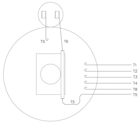
ALL CONNECTIONS ON STATIONARY SWITCH ARE SOLDERED
