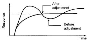
To stabilize response quickly, allowing for min. overshoot, : decrease the value of H23 I-gain or increase the value of
