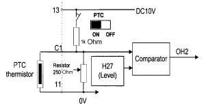
**Note:** Must be 0 setting when using 4-20mA reference or feedback signal and the PTC switch is off.
