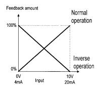
Only positive values can be input for this feedback amount of PID control. Negative values (e.g., 0 to -10V, -10 to 0V) cannot be input, thereby the function cannot be used for a reverse operation by an analog signal.
