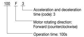
Set the operation time to 0.00 for any unused stages, which are skipped during operation.
