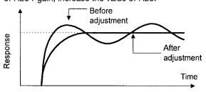
To suppress vibration with a frequency roughly equivalent to the value H24 D-gain, decrease the value of H24. If there is residual vibration with 0.0, decrease the value of H22 P-gain.
