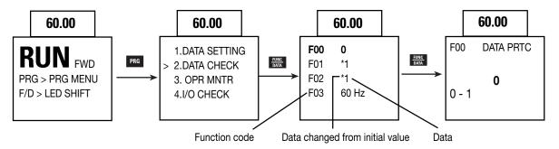
Select the desired function and press FUNC/DATA to check the function data. By pressing FUNC/DATA, the screen switches to the Data Setting screen, where data can be modified.
