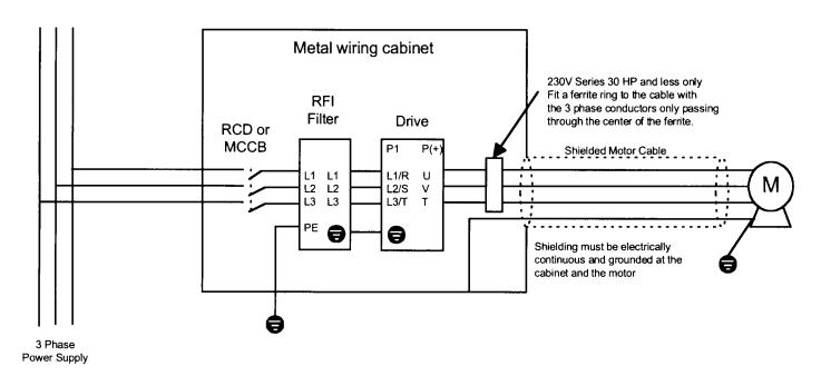
Figure 6 230V all Hp 460V less than 350 Hp
