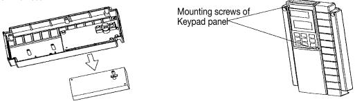
Fig.1-3-3 Removing the Keypad Panel (for drives of 30 HP or less)
