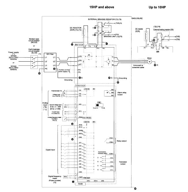
Note: The control circuit common terminals [11], (CM) and <CMY> are isolated
