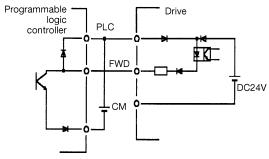
Fig. 2-3-11 Prevention of Bypass Current by External Power
