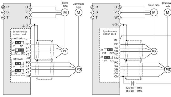
\* Pin J2 may be connected on either the 12V or 15V side.
