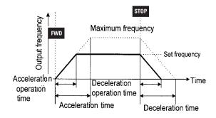
Note: If the set acceleration and deceleration times are set too low, even though the resistance torque and moment of inertia of the load are great, the torque limiting function or stall prevention function are activated. which prolongs the operation time beyond that stated above.
