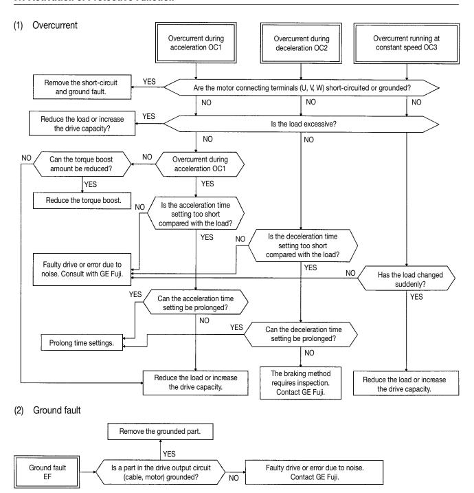
**Note:** The ground fault protective function is provided only for drive for nominal applied motors rated at 40 HP or more.
