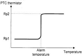
The figure above for H26 PTC thermistor (Mode select) shows that a 250W resistor and the thermistor (resistance value Rp) are connected in parallel. Hence, voltage Vc1 at Terminal C1 can be calculated using the following formula:
