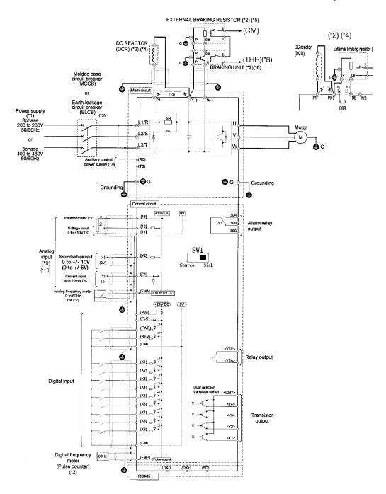
Note: The control circuit common terminals [11], (CM) and <CMY> are isolated
