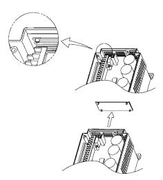
Fig. 2-2-4 Removing the ventilating cover
