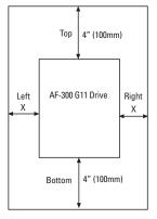
Fig. 2-2-1 30 HP or less: Gap X can be 0. (side-by-side installation) 40HP or more: Gap  $X >= 2.0^{\circ}$  (50mm)
