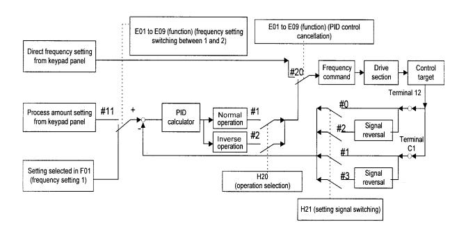
H22 PID control (P-gain)H23 PID control (I-gain)H24 PID control (D-gain)
