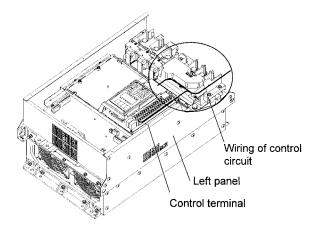
Fig. 2-3-12 The Control Wiring Route
