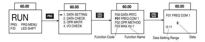
The function code consists of alphanumeric characters with unique letters assigned to each function group. Table 4-3-1
