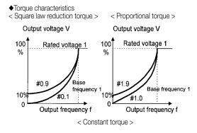
Since a large torque boost value creates over-excitation in the low-speed range, continued operation may cause the motor to overheat. Check the characteristics of the driven motor.
