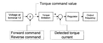
The torque command value is +200% when the voltage at Terminal 12 is +10V and is -200% when the voltage is -10V
