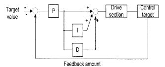
Forward or reverse operations can be selected for PID controller output. This enables motor revolutions to be faster or slower according to PID controller output.
