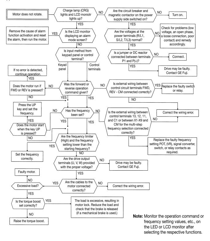
The motor does not rotate if the following commands are issued.
