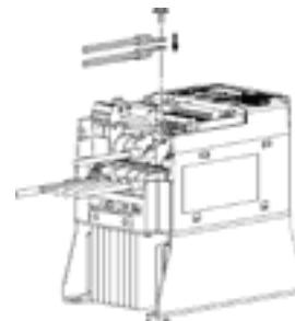
Figure 2.8 Braking Resistor Connection with DC Resistor
