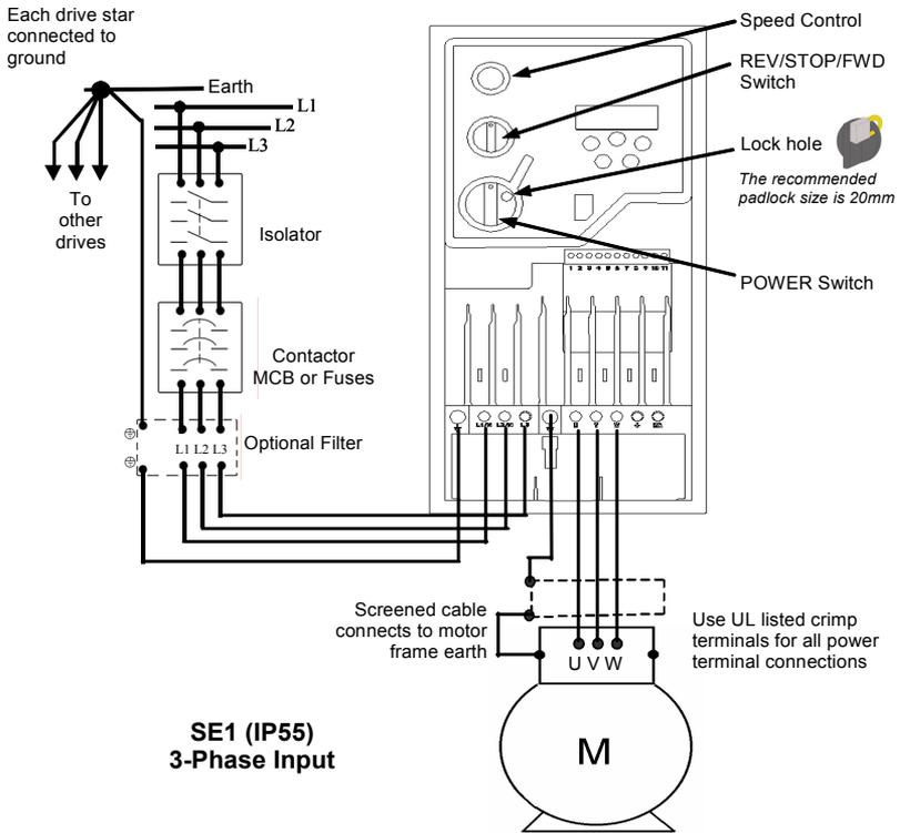
**Connecting the SE1 Microdrive, IP55 model**
