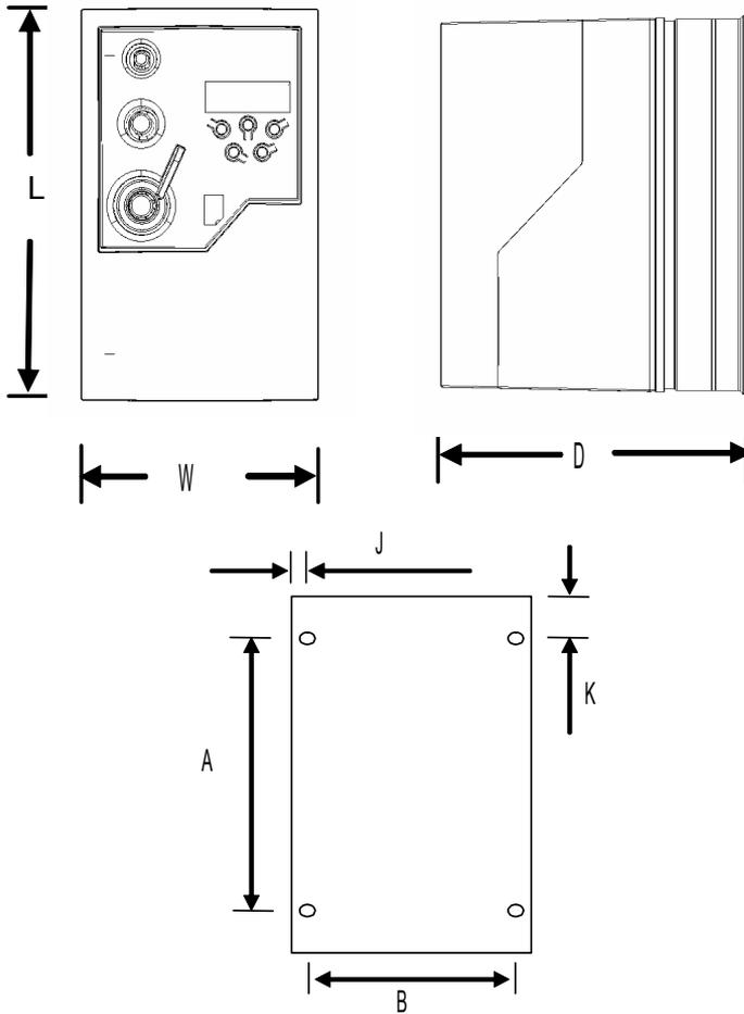
Mounting screws: **Size 1:** 2 x M4; **Size 2:** 4 x M4
