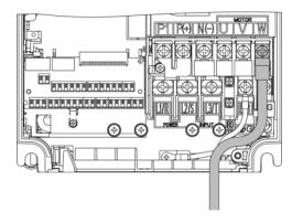
(9) For inverters of 900 and 1000 HP, two L2/S input terminals are arranged vertically to the terminal block. When connecting wires to these terminals, use the bolts, washers and nuts that come with the inverter, as shown below.
