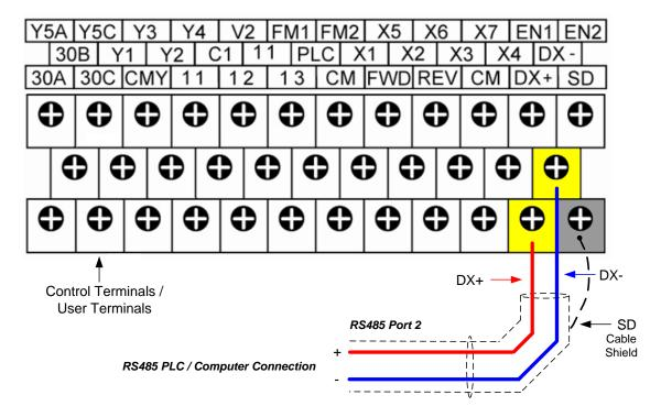
To Run/Stop (Operation Command) the EQ7 drive via serial communication parameter H30 has be set to either a "6" for Run/Stop via serial communication only or to "8" for Run/Stop (Operation Command) and Frequency Reference (Frequency Command).
