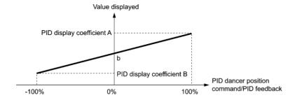
If the sensor output is unipolar, the PID dancer control operates within the range from 0 to +100%, so virtually specify the value at -100% as coefficient B.
