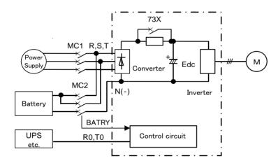
Figure A: Connection Diagram
