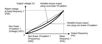
■ Torque boost: Data setting range: 0.0 to 20.0 (%) (100%/Rated voltage at base frequency)
