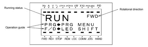
Figure 3.3 Display of Running Status
