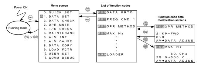
Figure 3.8 Configuration of Screens for "DATA SET"
