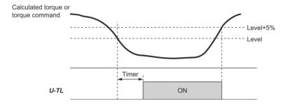
In the inverter's low frequency operation, as a substantial error in torque calculation occurs, no low torque can be detected within the operation range at less than 20% of the base frequency (F04). (In this case, the result of recognition before entering this operation range is retained.)
