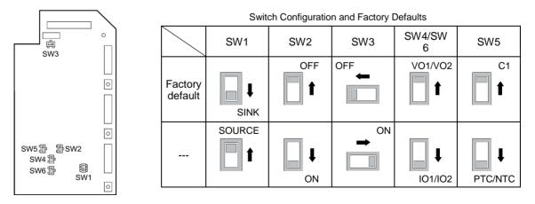
Figure 2.20 Location of the Slide Switches on the Control PCB
