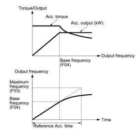
The figures at left show the acceleration characteristics. Similar characteristics apply to the deceleration.
