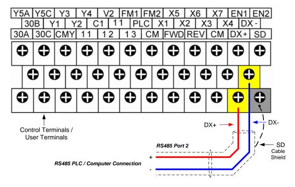
To set the speed reference for the EQ7 drive via serial communication parameter H30 has be set to either a "4" for frequency command via serial communication only or to "8" for Run Command and Frequency Reference (Frequency Command).
