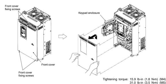
Figure 2.5 Removing the Front Cover (e.g. EQ7-4050-C)
