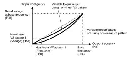
■ Torque boost Data setting range: 0.0 to 20.0 (%) (100%/Rated voltage at base frequency)
