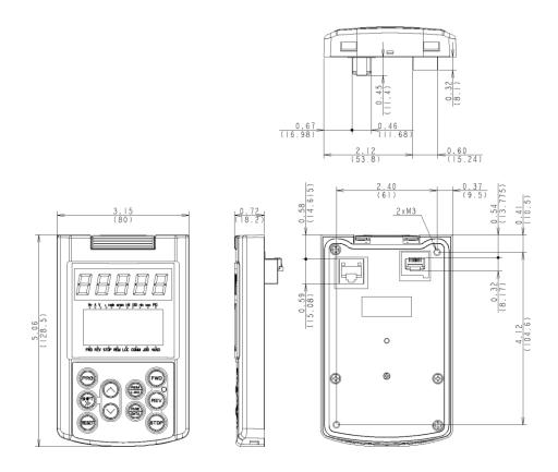
Drill four screw holes and cut a square hole in a panel as specified below.
