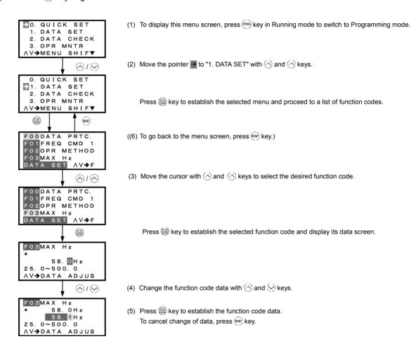
Figure 3.10 Screen Transition for "Data Checking"
