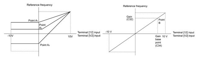
Configuring F18 (Bias) and C50 (Bias base point) to specify an arbitrary value (Points A1, A2, and A3) gives the bias as shown above.
