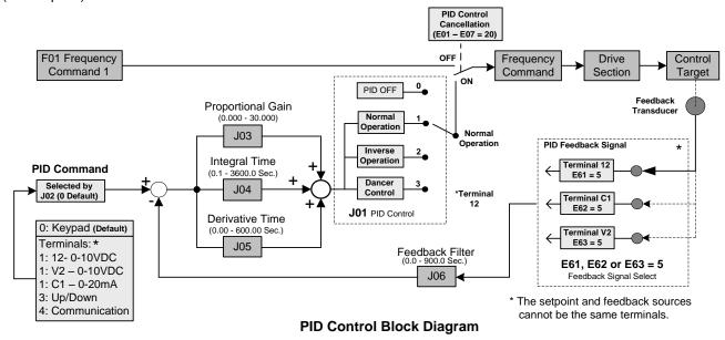
The amplitude of the error can be adjusted with the Proportional Gain parameter J03 and is directly related to the output of the PID controller, so the larger gain the larger the output correction.
