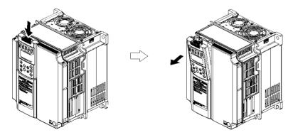
Figure 2.22 Removing the Keypad
