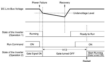
**Factory default:** By factory default, H13 is set to a matched value for the standard motor (see Table A in Section 5.1 "Function Code Tables"). Basically, it is not necessary to change H13 data. However, if the long restart time causes deteriorated performance or causes any other problem, reduce the setting to about a half of the default value, ensuring that no alarm occurs.
