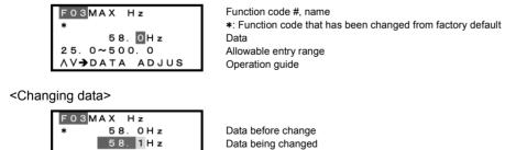
Figure 3.9 Screen Samples for Changing Function Code Data
