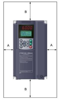
Figure 2.1 Mounting Direction and Required Clearances
