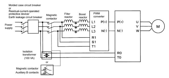
Figure 2.9 Connection Example of PWM Converter
