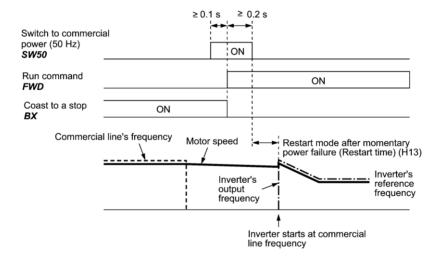
· When the motor speed decreases significantly during coast-to-stop (with the current limiter activated):
