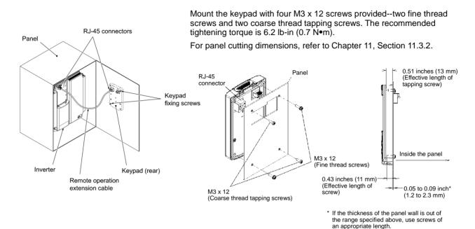
Figure 2.21 Mounting the Keypad on the Panel Wall
