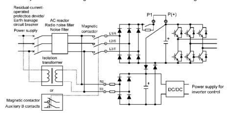
Figure 2.8 Connection Example of Residual-current-operated Protective Device (RCD)/ Earth Leakage Circuit Breaker (ELCB)
