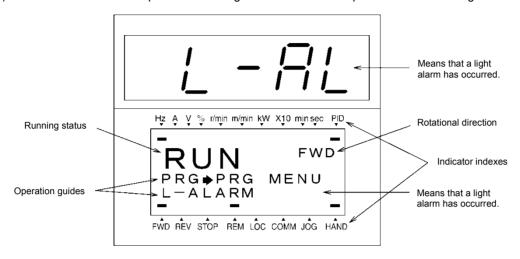
Figure 3.6 Display of Light Alarm
