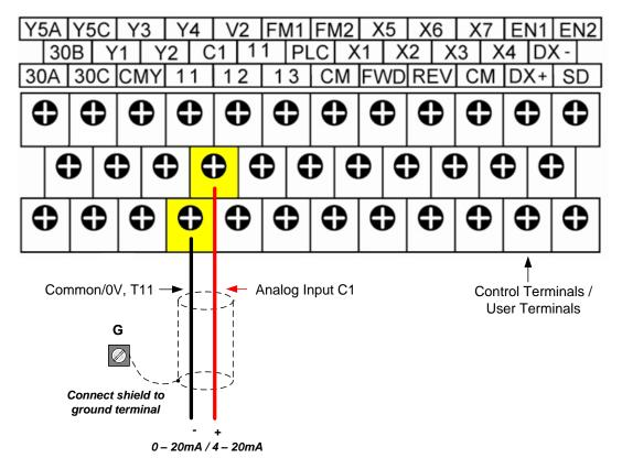
Note: When using a 0 – 20mA signal set parameter C40 to 1.
