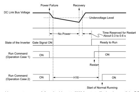
If H16 (Allowable momentary power failure time) is set to "999," restart will take place until the DC link bus voltage drops down to the minimum allowable voltage for restart after a momentary power failure (50 V for 230 V series and 100 V for 460 V series). If the DC link bus voltage drops below the allowable voltage, the inverter recognizes that the power has been shut down and does not restart.
