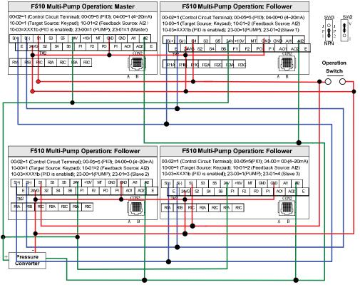
**Multi-Pump Wiring Diagram**
